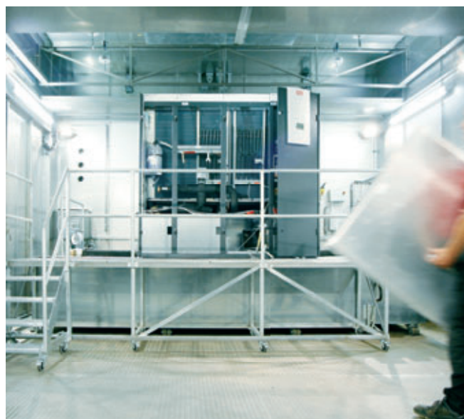
Interior dimensions of the climatic chamber: Height 4180 mm, width 9760 mm, depth 5680 mm
